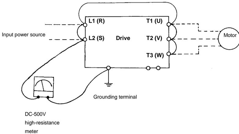
**Connection for dielectric strength test**
