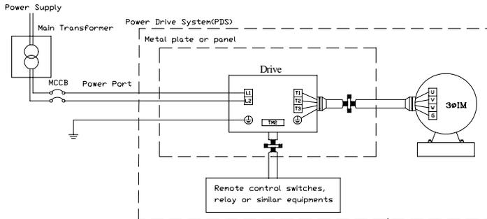
When the distance between the inverter and motor is longer than 100 meters, cable wire should be carefully chosen to reduce the wiring resistance below 3% and the voltage drop
