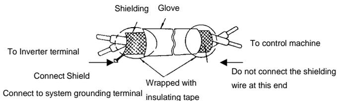
(C) The grounding terminal of the inverter must be correctly grounded in compliance with 200V class type three grounding.
