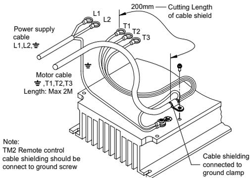
**SYN10 S 220 01/03/05 IP65 S (NEMA4) (WITH SWITCH TYPE) EMC MOUNTING & CONNECTIONS:**
